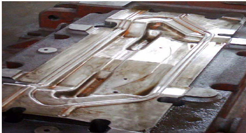
Figure 1. A drawing die of the corner backstop of the front floor of a truck.
